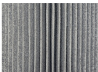
Figure 3: Filter cartridge after cleaning with compressed air
