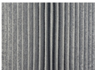
Figure 3: Filter cartridge after cleaning with compressed air
