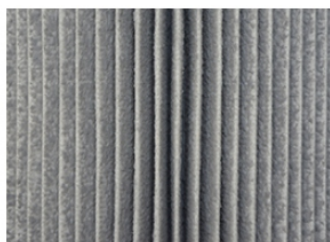
Figure 3: Filter cartridge after cleaning with compressed air
