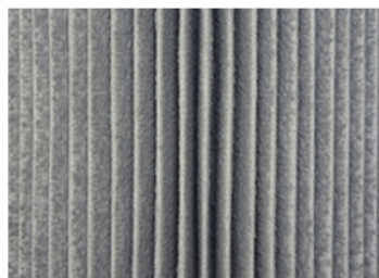
Figure 3: Filter cartridge after cleaning with compressed air
