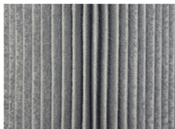
Figure 3: Filter cartridge after cleaning with compressed air
