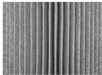
Figure 3: Filter cartridge after cleaning with compressed air
