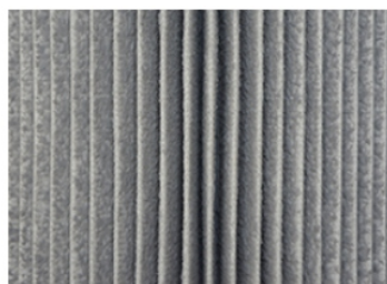
Figure 3: Filter cartridge after cleaning with compressed air
